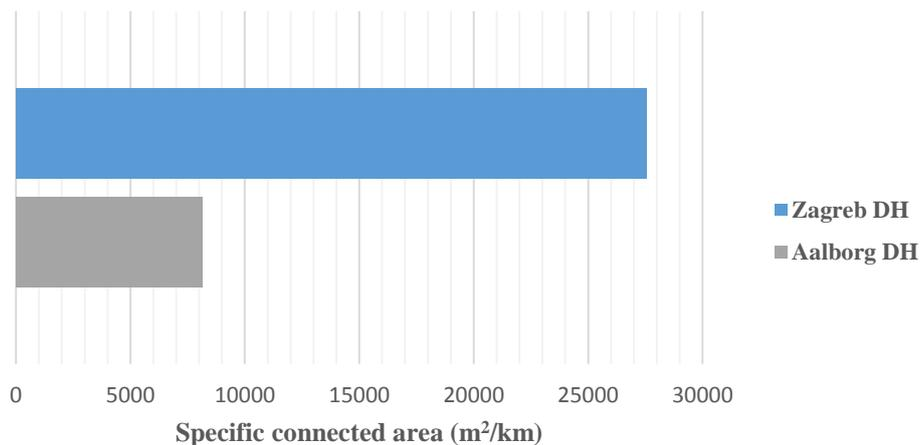
**Figure 42. Specific connected area per km of DH network length**
