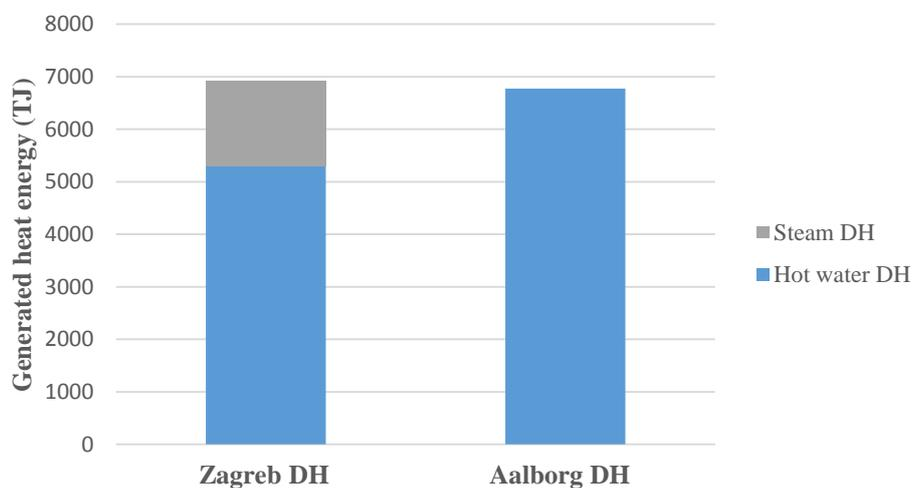
**Figure 26. Distribution of generated heat energy to hot water and steam DH**
