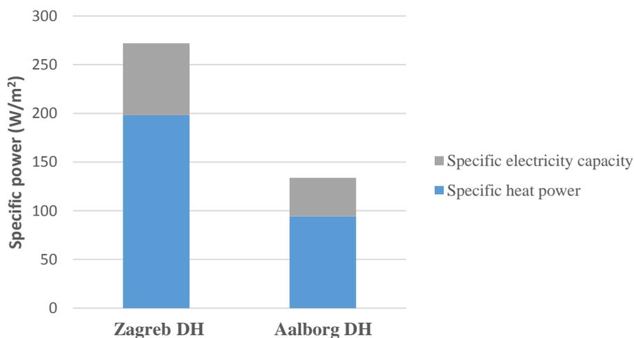
**Figure 31. Specific heat power and specific electricity capacity per connected area**
