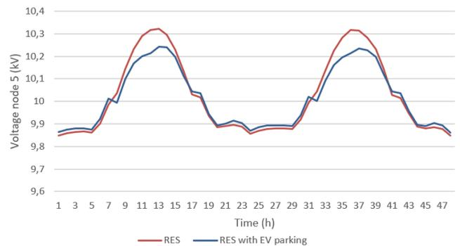
Figure 19. Voltage at node 5 for RES scenario
