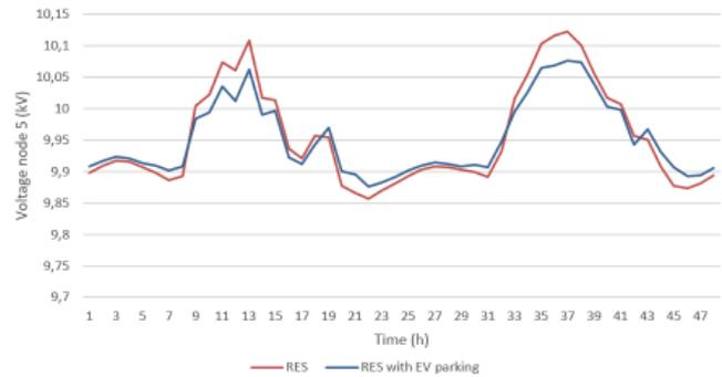
Figure 25. Voltage at node 5 during February for RES scenario
