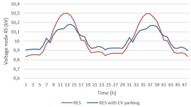
Figure 17. Voltage at node 45 during July for RES scenario
