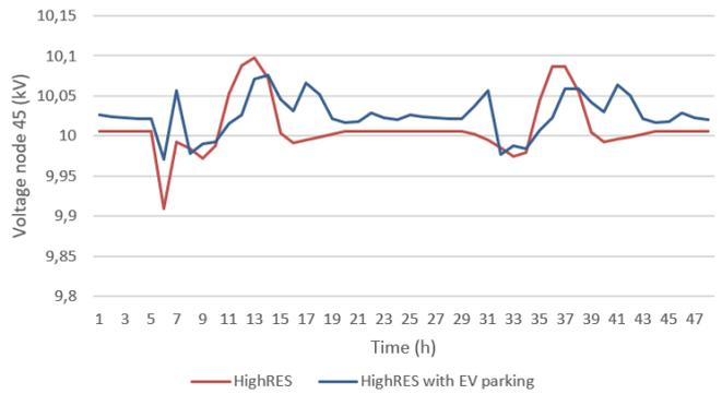
Figure 18. Voltage at node 45 during July for HighRES scenario
