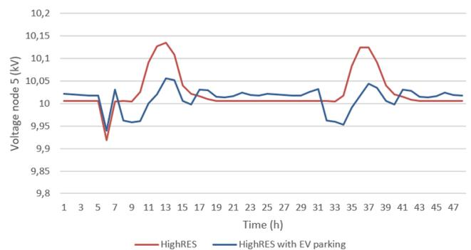
Figure 20. Voltage at node 5 for HighRES scenario
