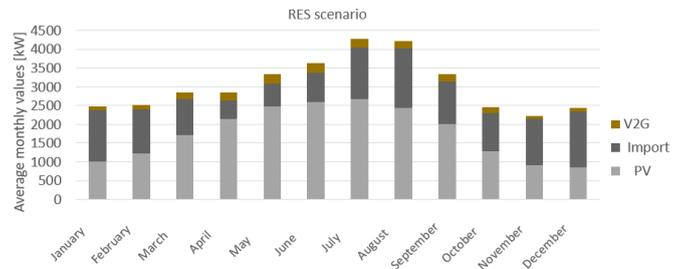
Figure 5. Results of RES scenario as monthly average hourly production of electricity
