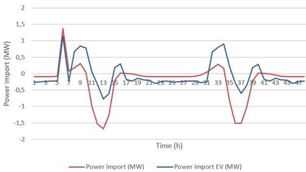
Figure 16. Power import during July for HighRES scenario
