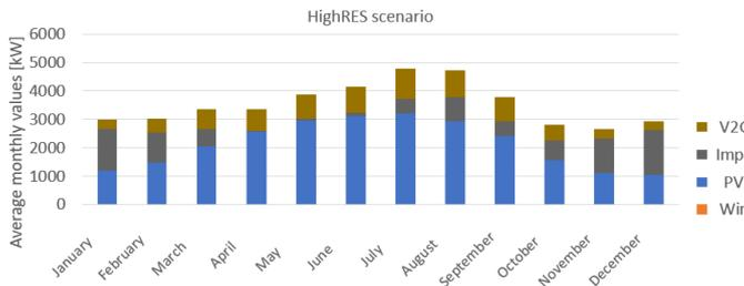
**Figure 8.** Results of "HighRES" scenario as monthly average hourly production of electricity
