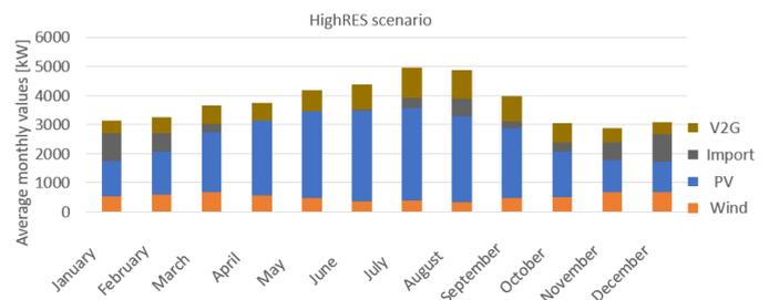
Figure 6. Results of "HighRES wind" scenario as monthly average hourly production of electricity
