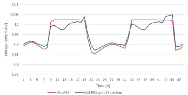
Figure 26. Voltage at node 5 during February for HighRES scenario
