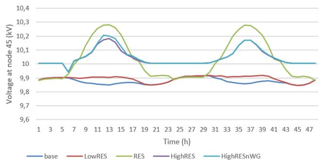
**Figure 10.** Voltage variation at node 45 during two days in July
