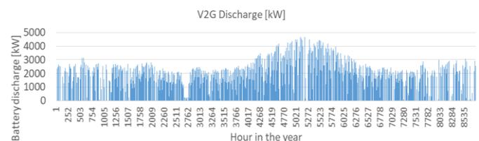
Figure 7. Discharge from electric vehicle batteries
