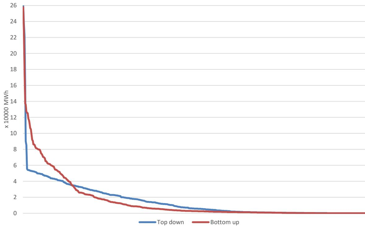
Figure 7 Distribution curve of top down and bottom up heat demand
