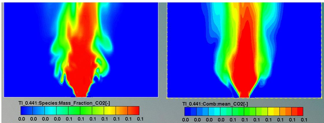
Figure 54 - Instantaneous and mean CO2 mass fraction
