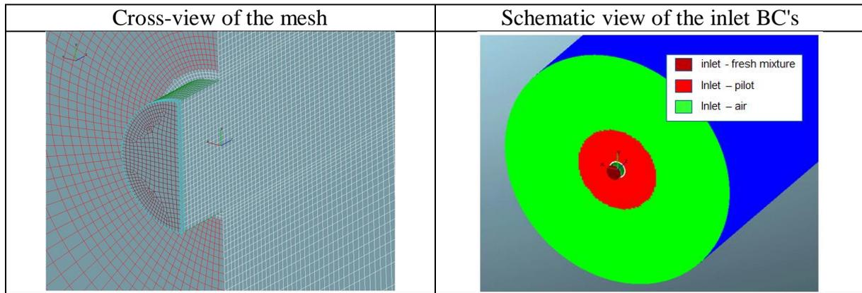
Figure 25 - Mesh and inlet configuration for Chen case.
