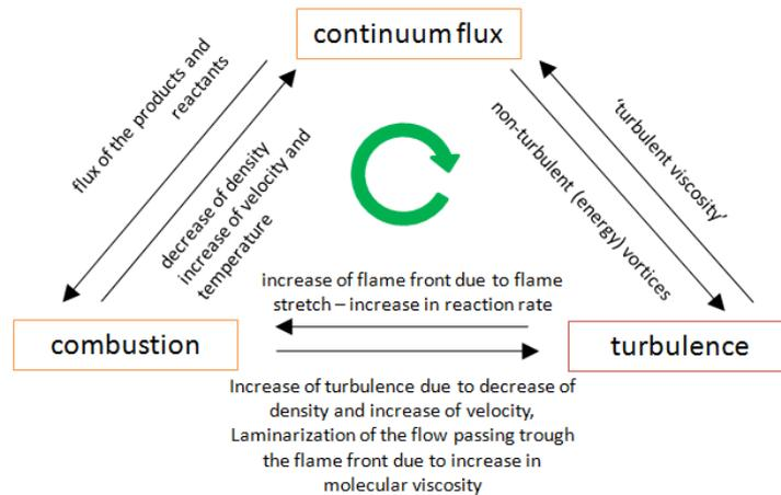
Figure 1 - Schematic representation of turbulence-flame interaction.
