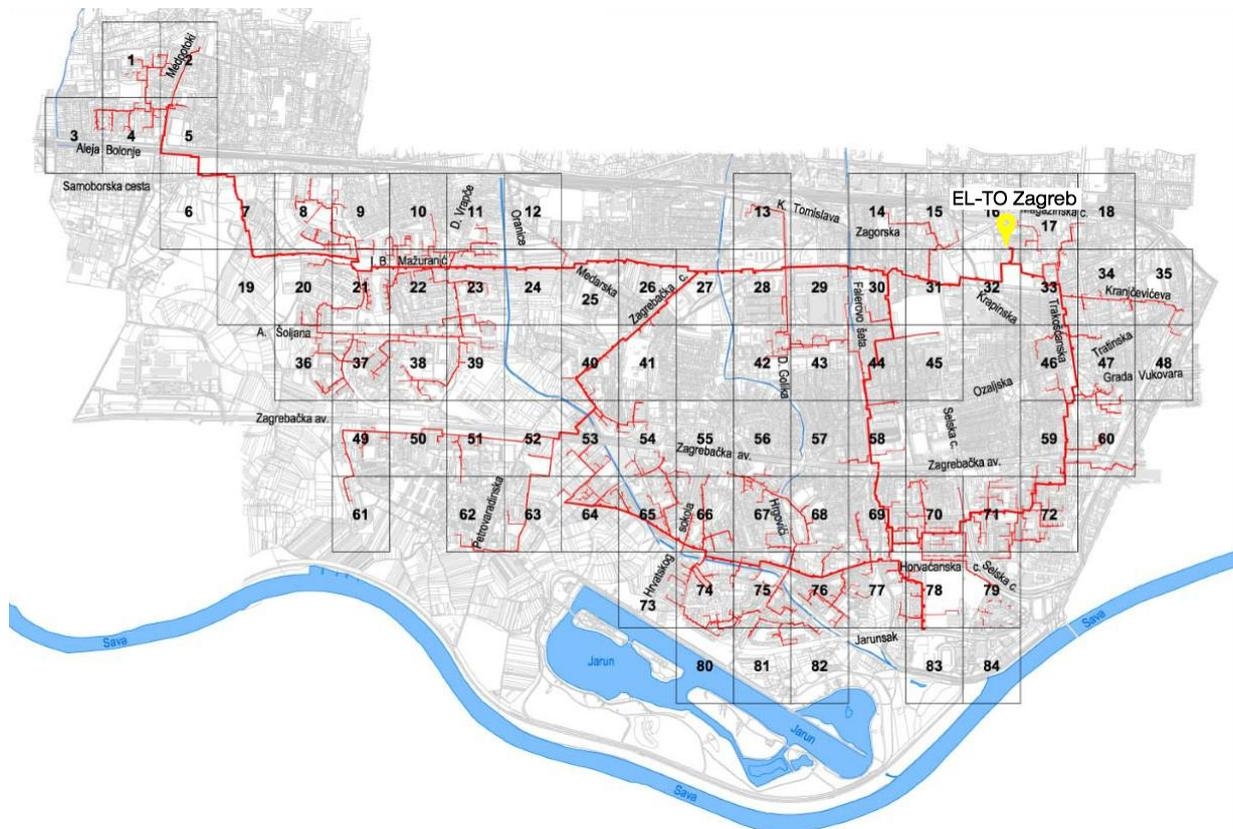
Figure 34. Network structure of district heating area „West“ [28]
