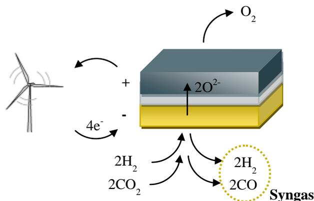
Figure 27. Solid oxide cell co-electrolysis
