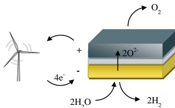
Figure 25. Solid oxide cell water electrolysis
