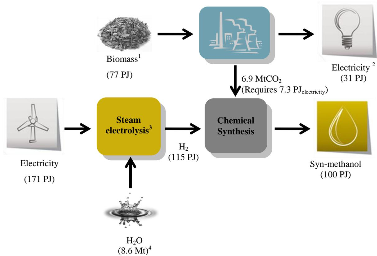
Figure 31. <sup>1</sup>Based on dry willow biomass. <sup>2</sup>Assumed an electricity generation efficiency of 40%. <sup>3</sup>Assumed an electrolyser efficiency of 73% [12], minus 5% account for storage and chemical synthesis losses. <sup>4</sup>This does not include the excess water which can be recycled from the hydrogenation process.
