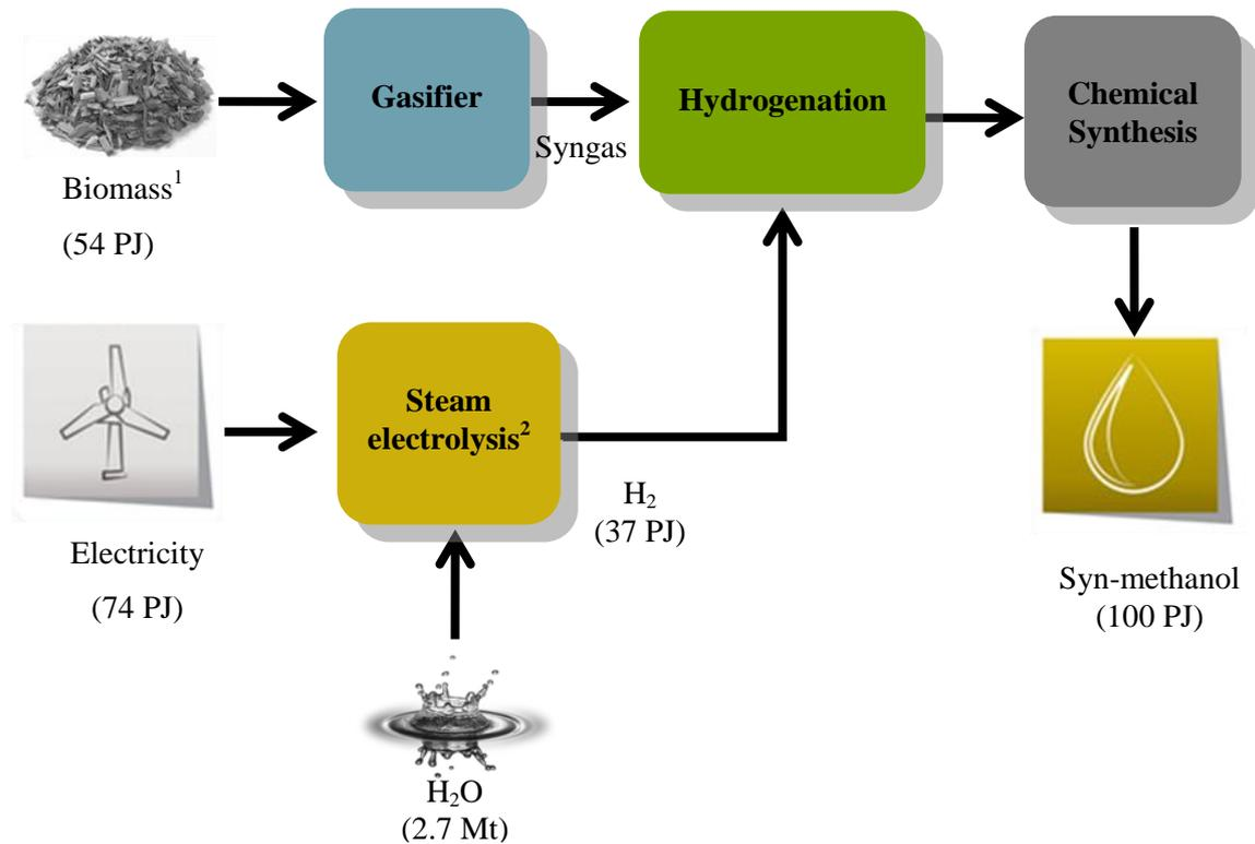
Figure 32. Gasification of biomass. <sup>1</sup>Based on straw/wood chips. <sup>2</sup>Assumed an electrolyser efficiency of 73% [12], minus 5% account for storage and chemical synthesis losses.
