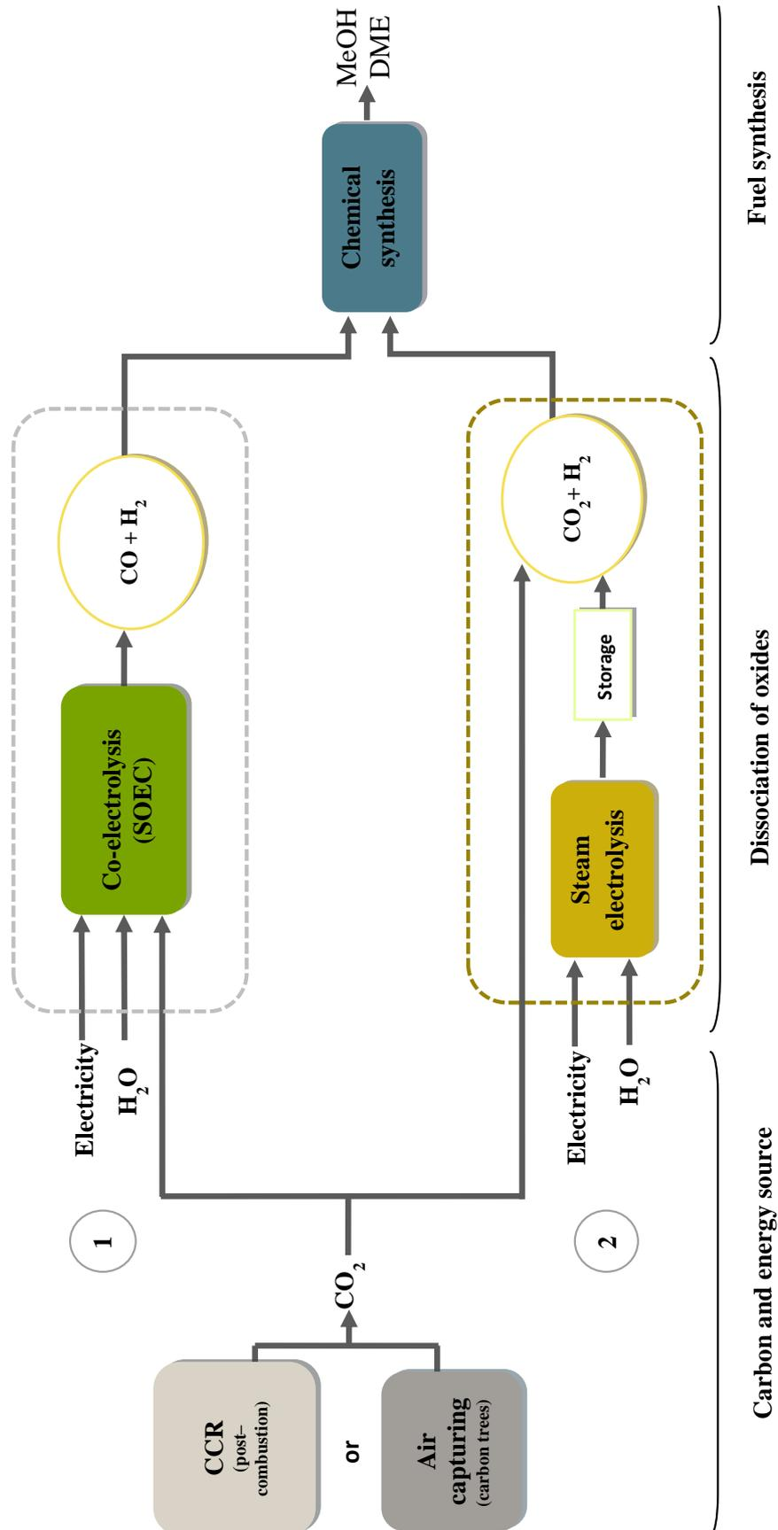
Figure 28. Pathways for production synthetic methanol or DME, first *co-electrolysis*, second  $\text{CO}_2$  *hydrogenation*
