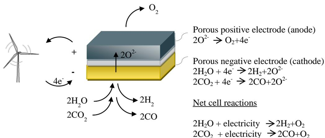
Figure 16. Electrolysis reactions
