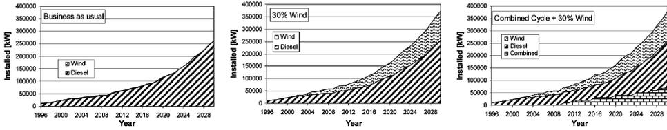
Fig. 2. Installed capacity for three scenario—wind does not reduce significantly the installed diesel capacity needed.
