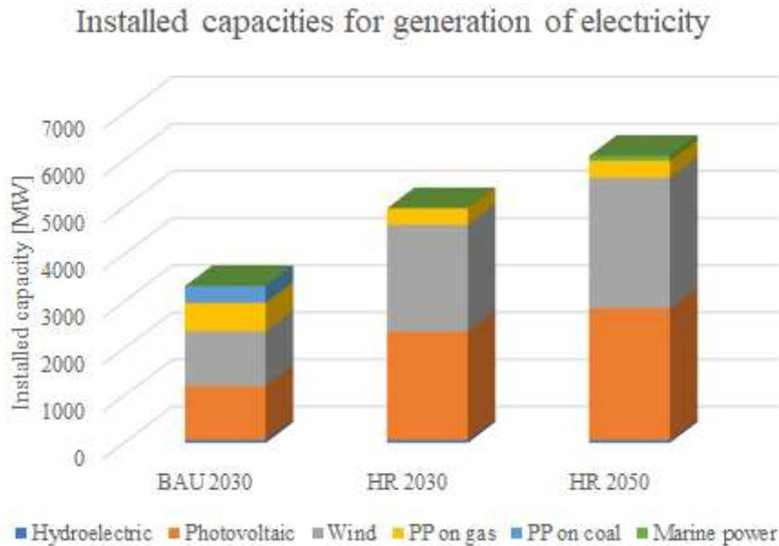
Figure 5. The installed capacity by type of plant in future scenarios
