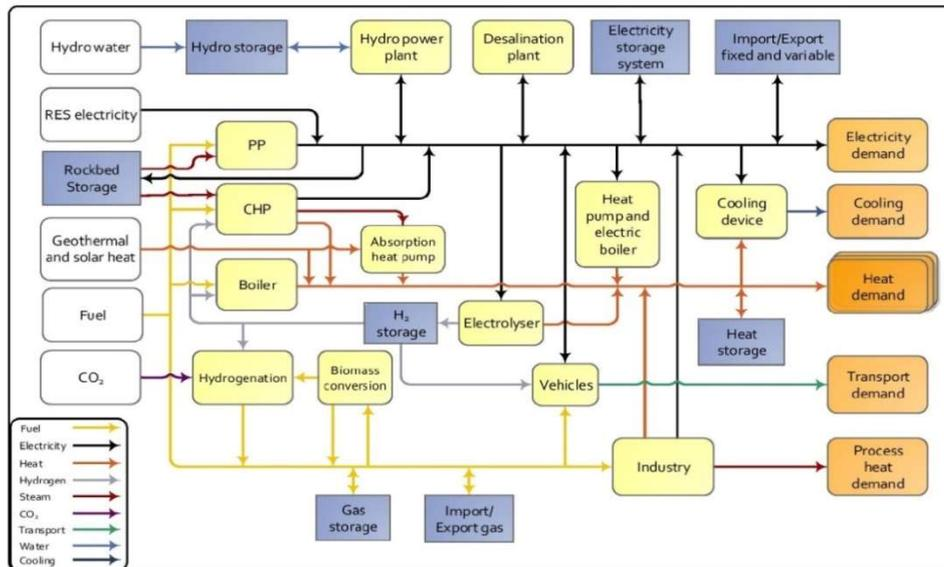
Figure 1 Schematic diagram of the EnergyPLAN model [20]
