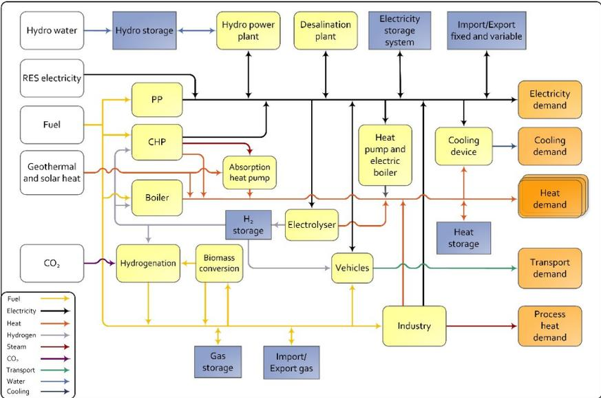
Figure 1 Principal scheme of energy system in EnergyPLAN
