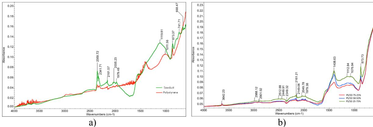
Figure 7. - FTIR spectra of char from a) individual pyrolysis, and b) respective blends
