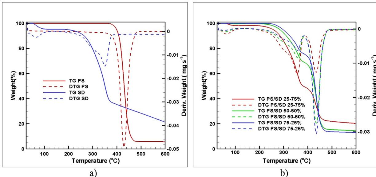
Figure 2. - TG curves for individual biomass and PS samples (a) and their respective mixtures (b)
