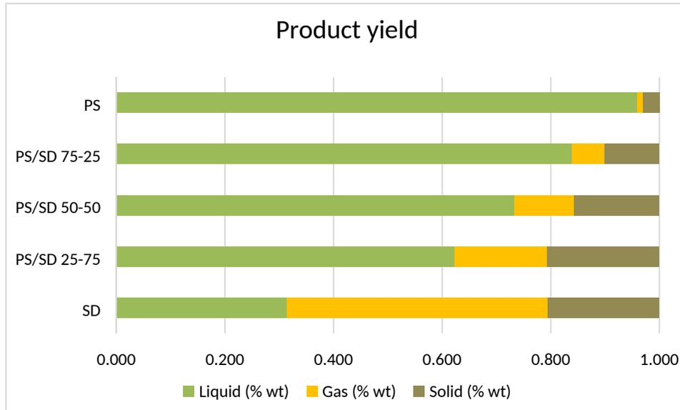
Figure 3. - Product yield from individual pyrolysis and PS/SD blends co-pyrolysis
