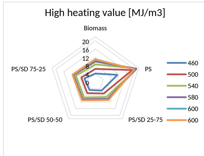
Figure 6. - Calculated HHV for obtained syngas compositions
