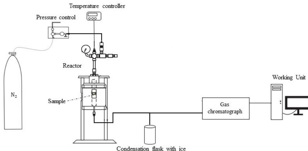
Figure 1 – Experimental setup used for the pyrolysis and co-pyrolysis of investigated samples
