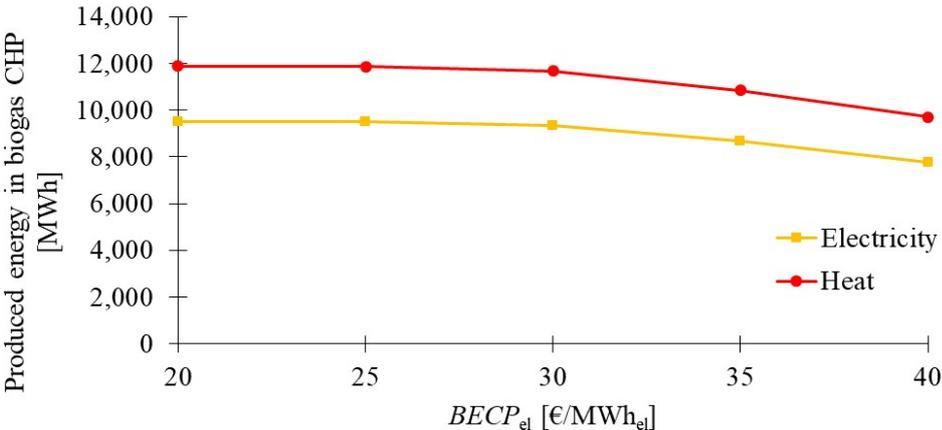
Figure 4 Energy produced in biogas CHP, Scenario I)
