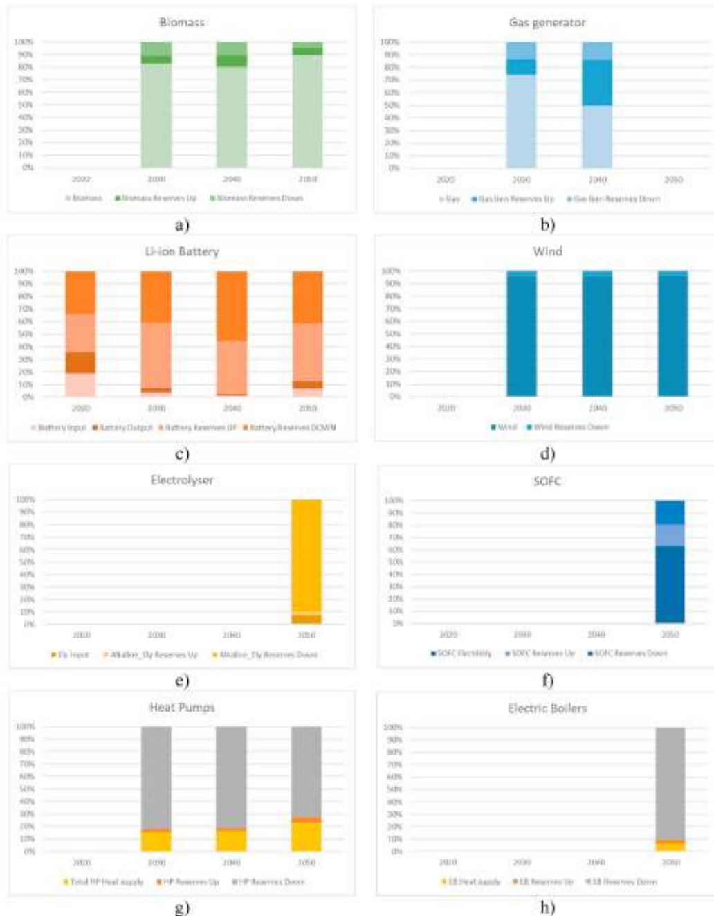
Fig. 10. Percentage of type of use for main reserve provider technologies: a) Biomass generator; b) Gas generator; c) Li-ion battery; d) Wind turbine; e) Electrolyser; f) Solid-Oxide Fuel Cell; g) Heat Pumps; h) Electric Boilers.
