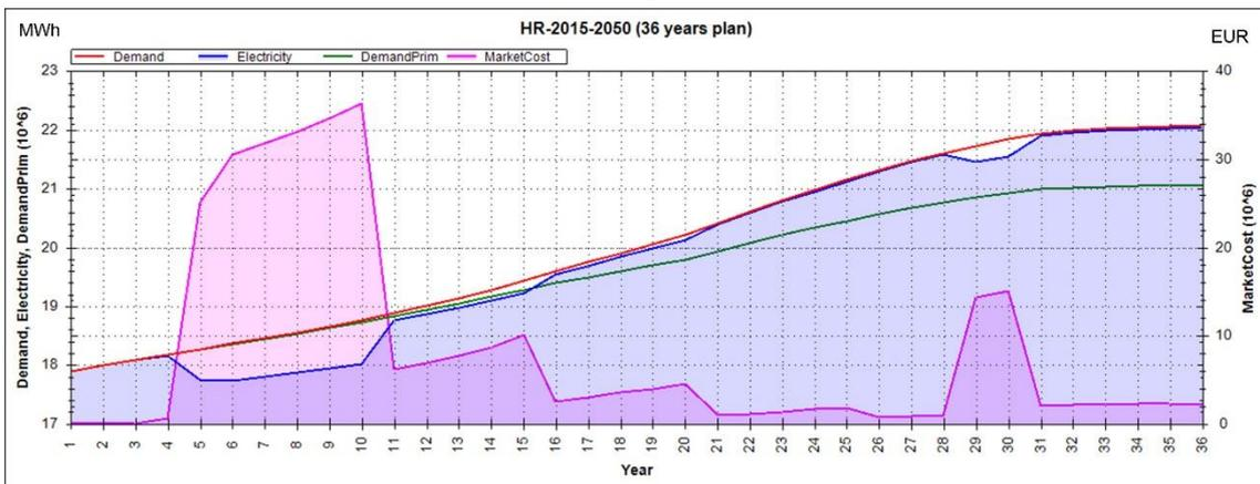
Figure 15. Design B – Cumulative Primary and Total Demand, Produced and Purchased Electrical Energy
