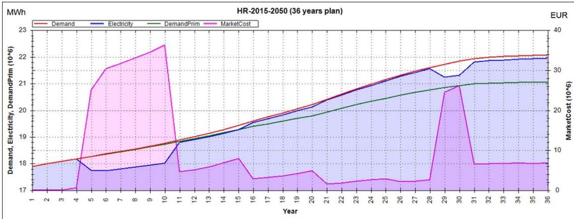
Figure 13. Design A – Cumulative Primary and Total Demand, Produced and Purchased Electrical Energy
