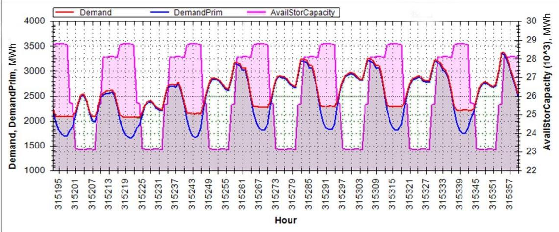
Figure 9. H2RES modelled of primary electrical demand, total demand with energy for EV transport, and available capacity for use in energy system
