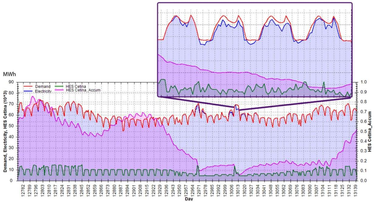
Figure 18. Design A – Last year Cumulative Demand, Total Electrical Energy, Hydro Energy and Accumulation
