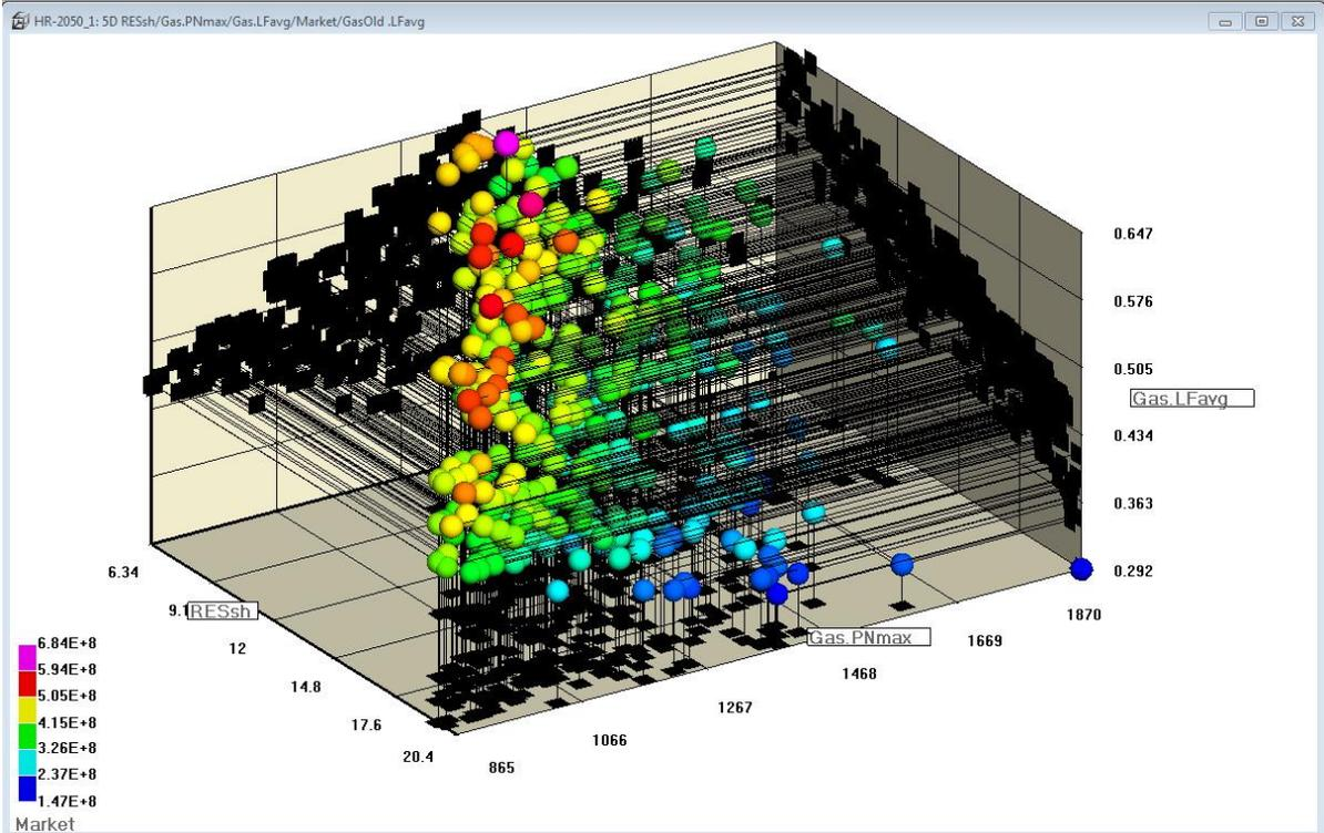
Figure 12. Relation between RES share, total installed nominal power of new Gas power plant with district heating and its load factor
