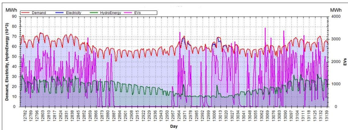
Figure 17. Design A – Last year Cumulative Demand, Total Electrical Energy, Hydro and EV Energy
