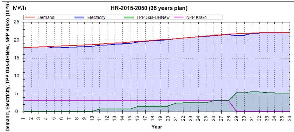
Figure 16. Design B - Cumulative Primary and Total Demand, NPP Krsko and new DH GAS Powerplant
