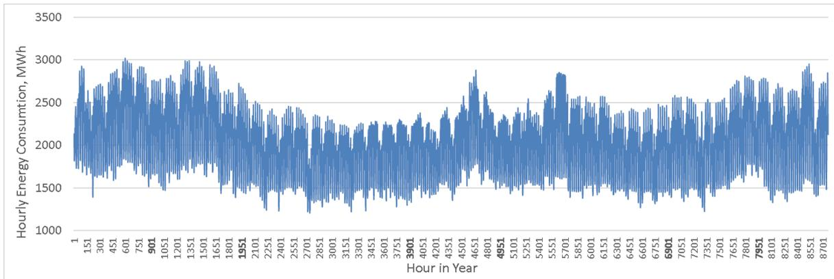
Figure 5. Anticipated electrical energy consumption for CES in 2015 (scenario starting year)
