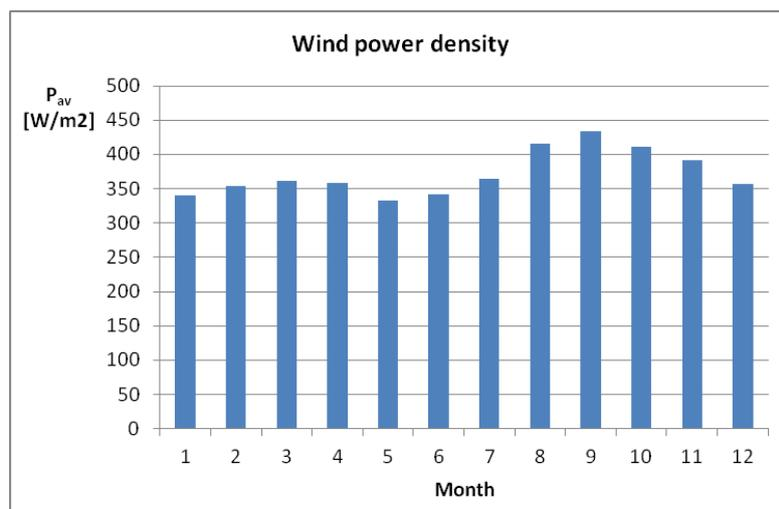
Figure 2. Wind power density averaged by month over the 30-year time span, to the height of 2500 meters and over the available region.
