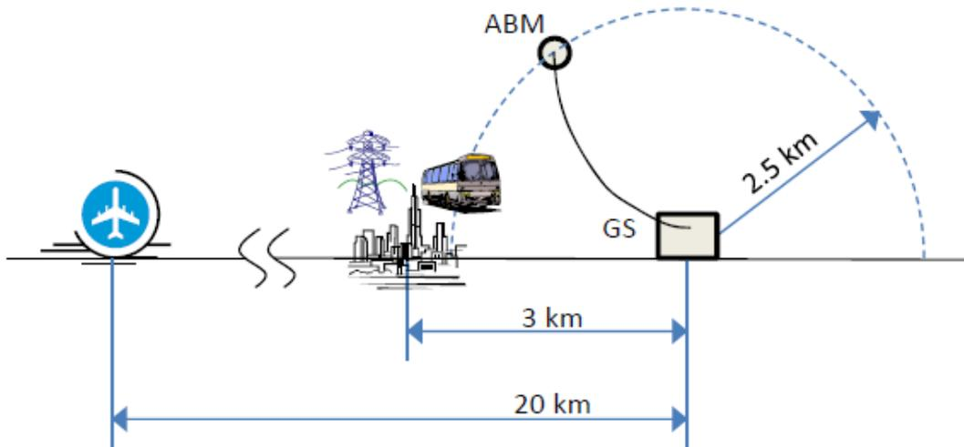
Figure 1. Schematic view of the safety concept in the case of systems utilizing high altitude wind energy.
