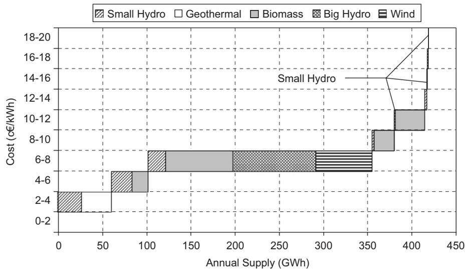
Fig. 8. RES cost-supply curve for 2006 (GW h).
