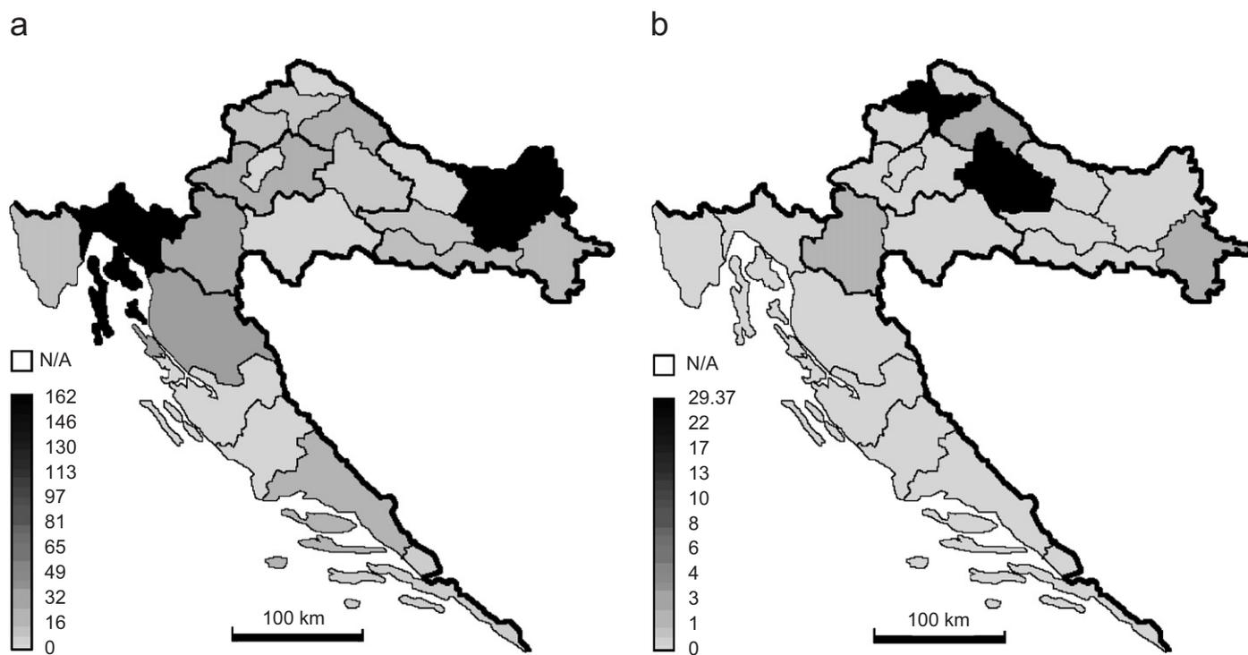
Fig. 6. (a) Energy capability of potential biomass facilities (GWh) and (b) maximum load capacity of potential geothermal facilities (MW).
