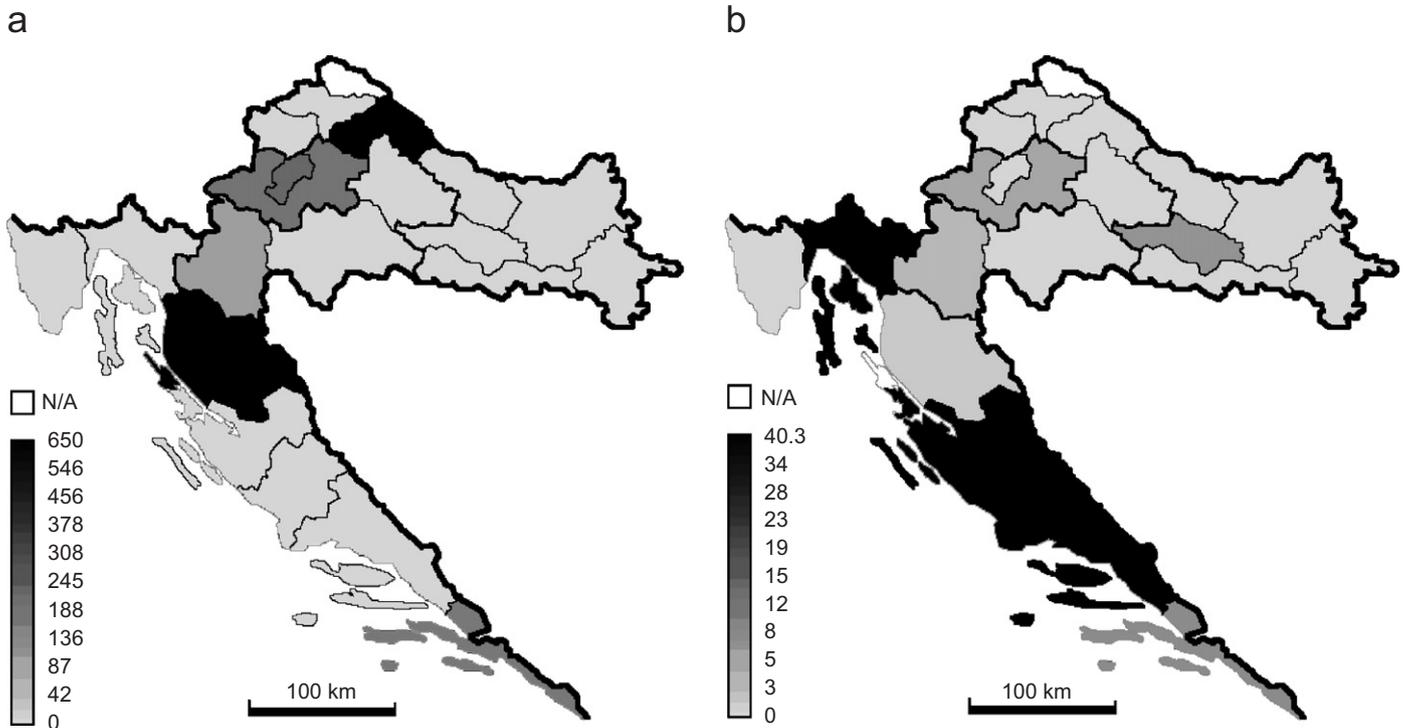
Fig. 7. Energy capability (GWh) of potential: (a) large and (b) small hydro power plants.
