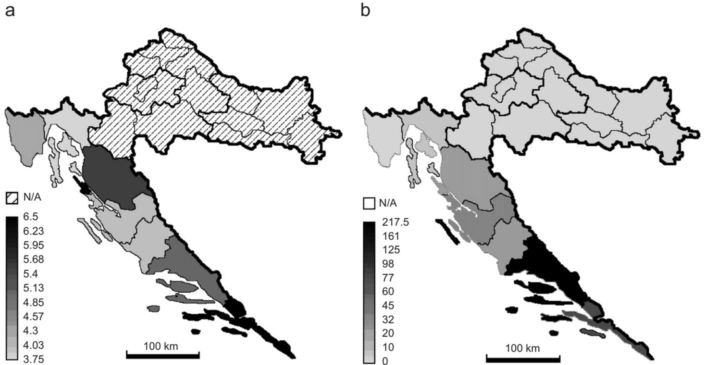
Fig. 3. (a) Average annual wind velocity (m/s) and (b) maximum load capacity of proposed wind facilities (MW).
