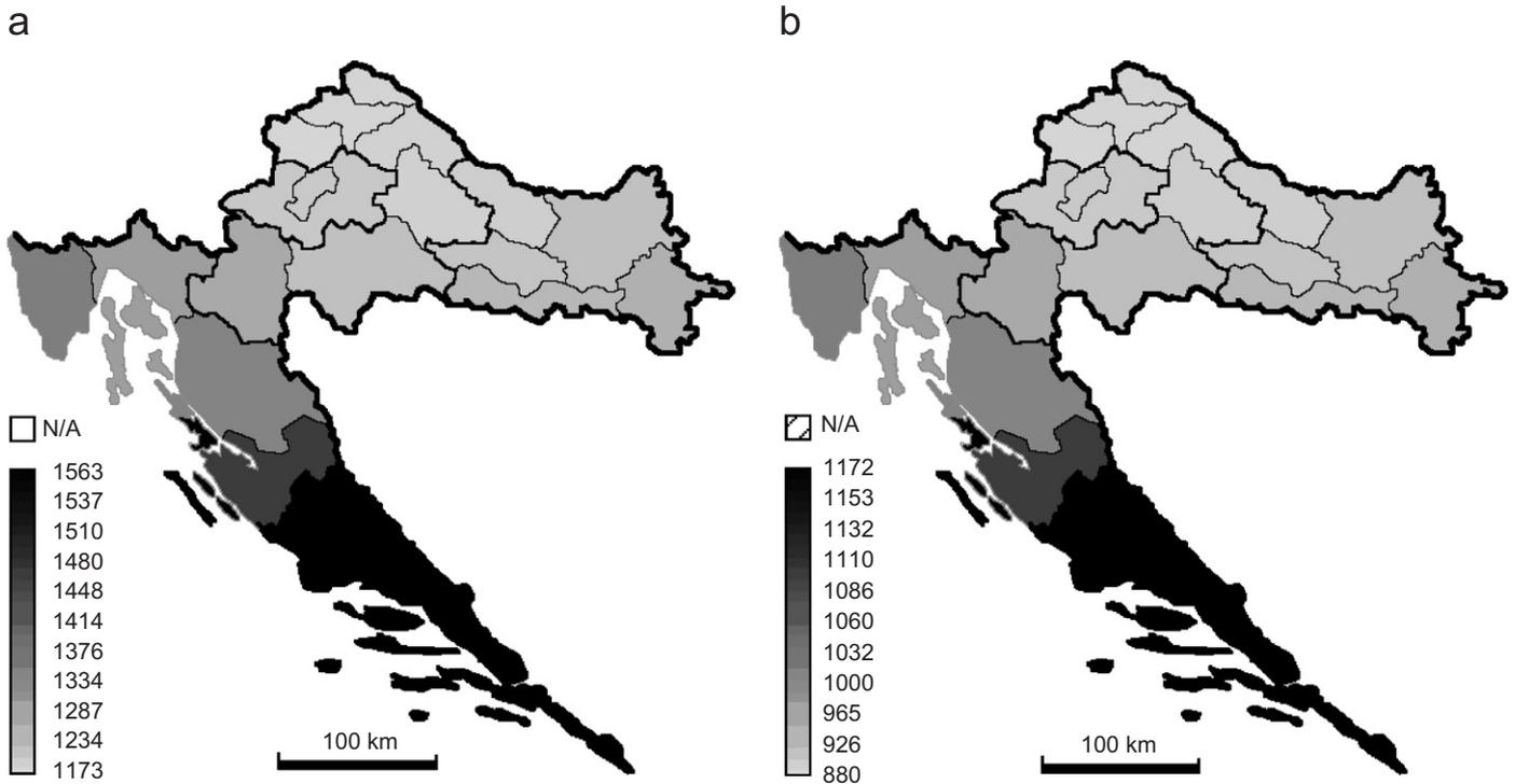
Fig. 2. (a) Global horizontal irradiation (kWh/m<sup>2</sup>/year) and (b) PV power (horizontal) (kWh/year for 1 kWp).
