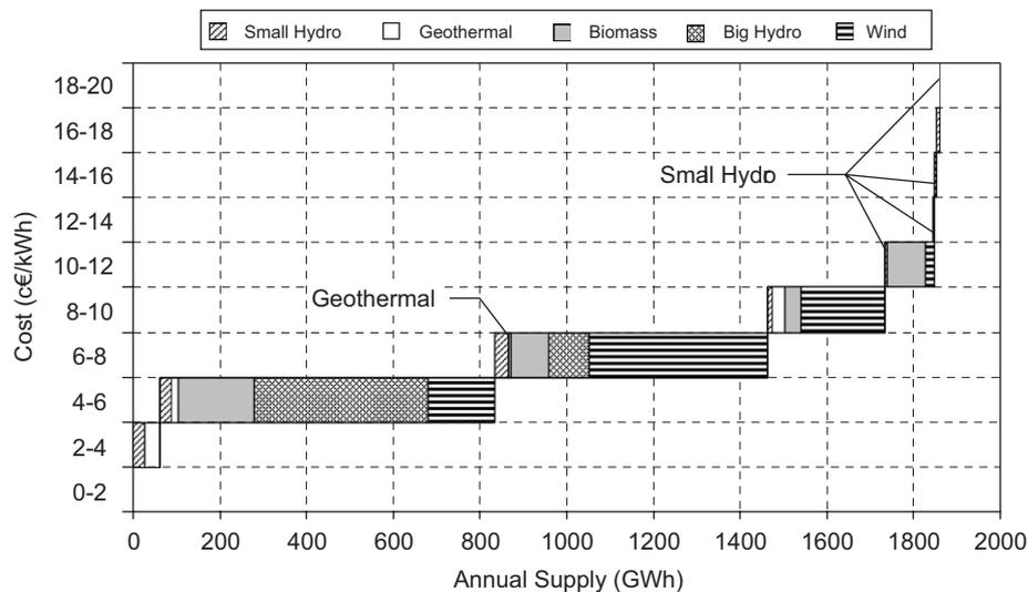
Fig. 9. RES cost-supply curve for 2010 (GW h).
