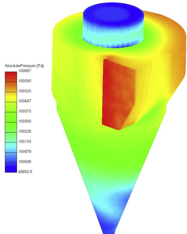
Fig. 8. 3-D view of the cyclone's absolute pressure distribution.
