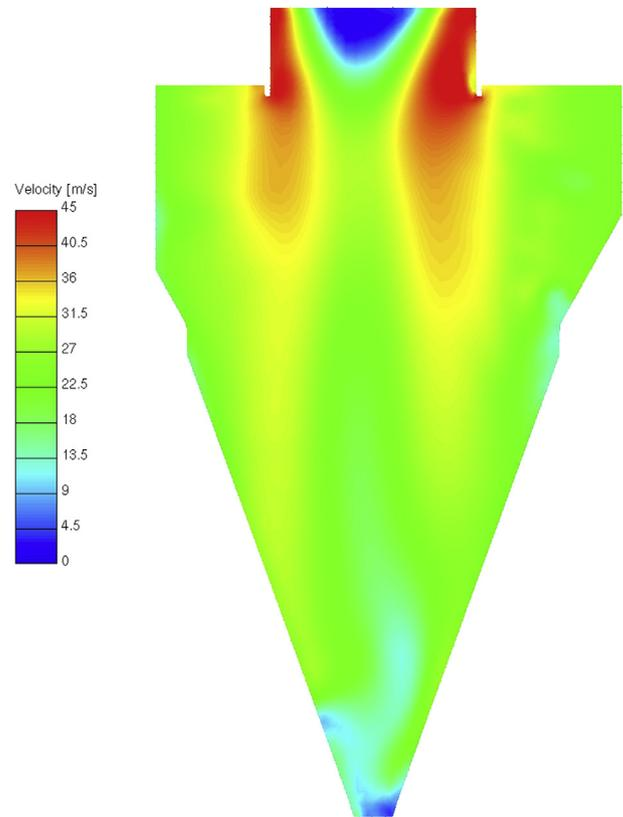
Fig. 4. Velocity field inside the calculated cyclone.
