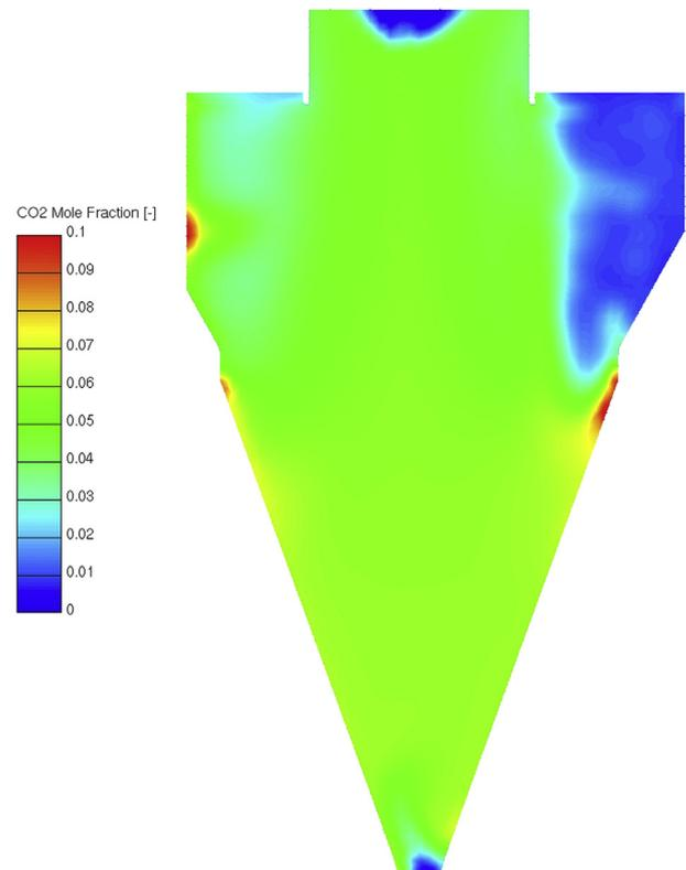
Fig. 5.  $\text{CO}_2$  mole fraction inside the calculated cyclone.
