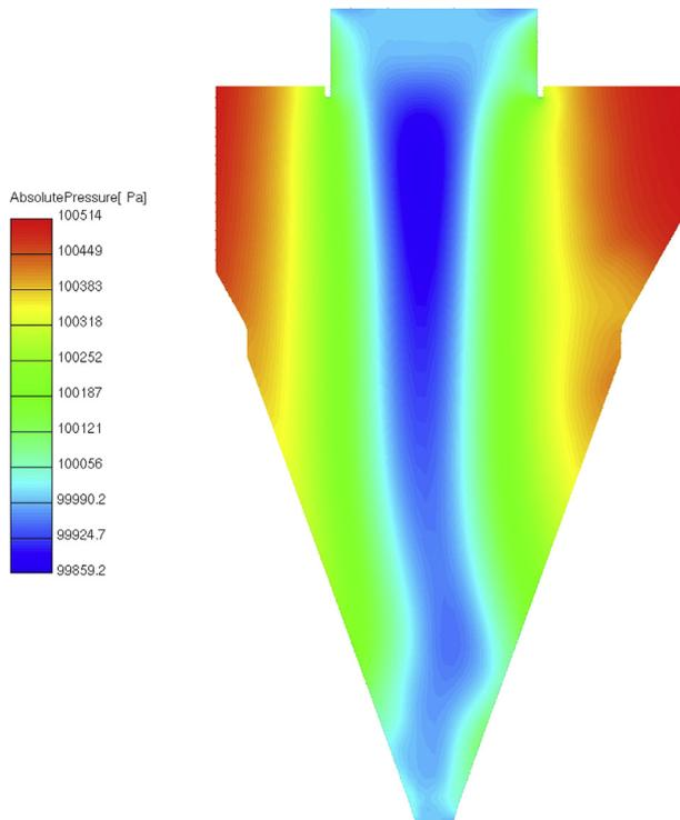
Fig. 3. Absolute pressure inside the calculated cyclone.
