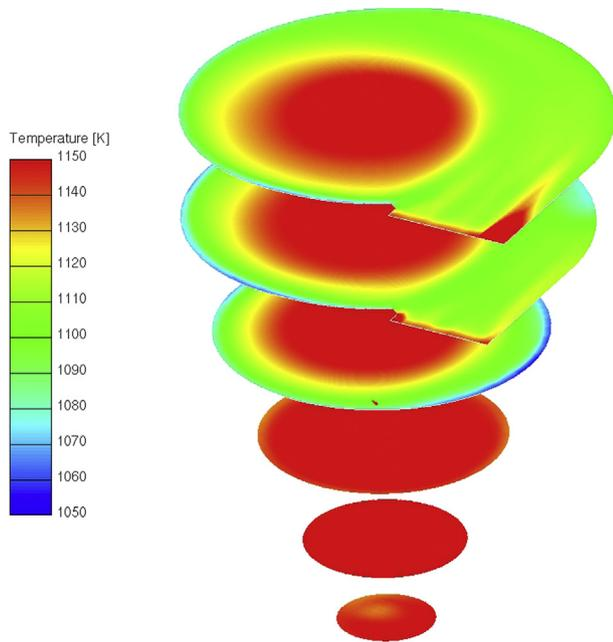
Fig. 9. Temperature field inside the calculated cyclone.
