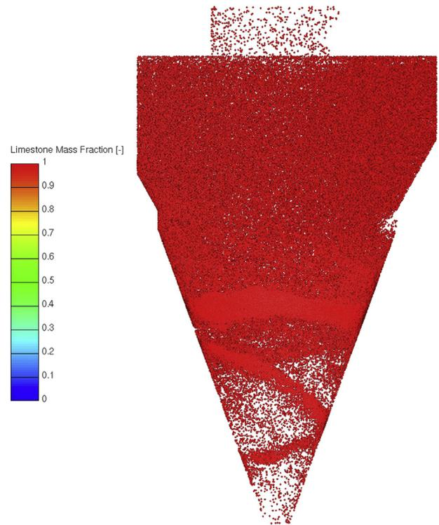
Fig. 7. Calcination process inside the calculated cyclone.
