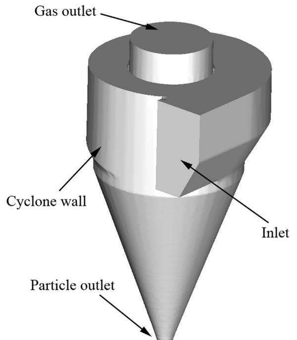
Fig. 1. Cement cyclone's geometry and boundary conditions.
