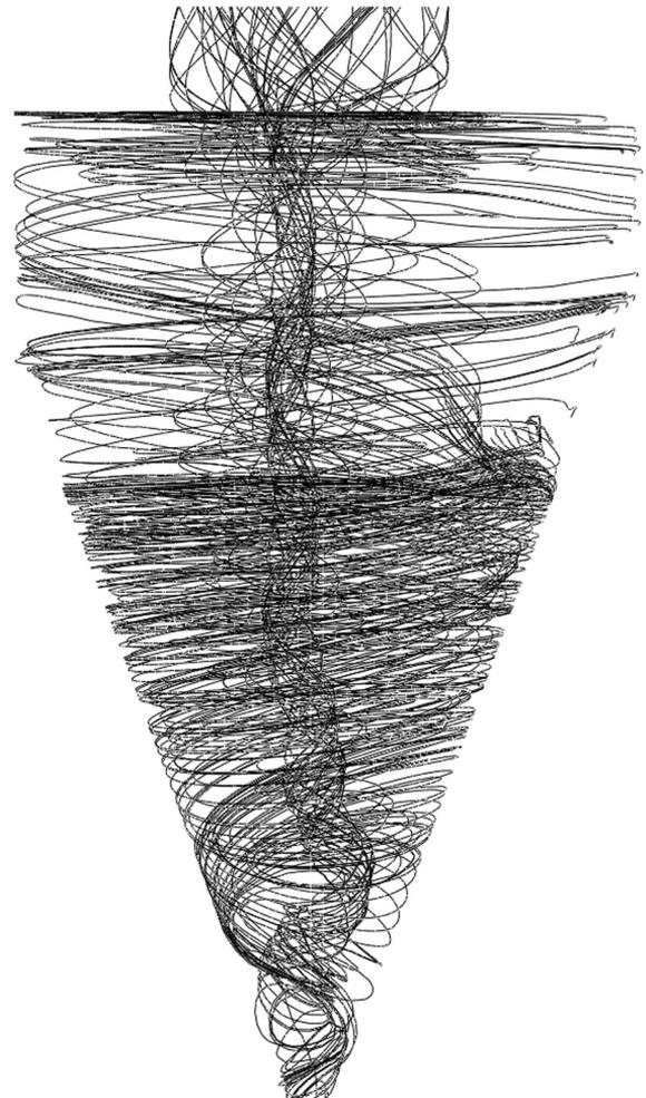
**Fig. 2.** Flow streamlines inside the calculated cyclone.
