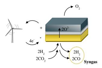
Figure 27. Solid oxide cell co-electrolysis
