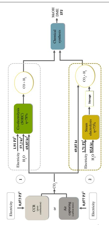
Figure 29. Methanol/DME synthesis from carbon capture and recycling/Air capturing. <sup>1</sup>Energy required for extracting 69.85 kt CO<sub>2</sub> calculated from [69]. <sup>2</sup>Energy required calculated according to [58]. <sup>3</sup>Electricity needed for both electrolysis processes is calculated according to efficiency and methanol/hydrogen ratio. <sup>4</sup>Water and CO<sub>2</sub> masses are calculated from mass balances for 1 PJ of methanol.
