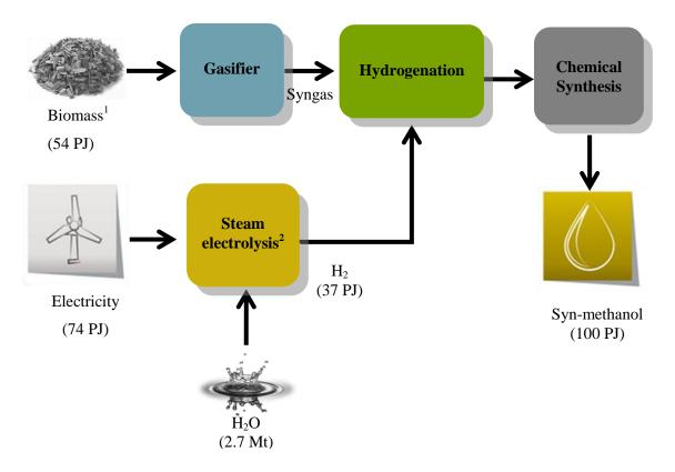
Figure 32. Gasification of biomass. <sup>1</sup>Based on straw/wood chips. <sup>2</sup>Assumed an electrolyser efficiency of 73% [12], minus 5% account for storage and chemical synthesis losses.
