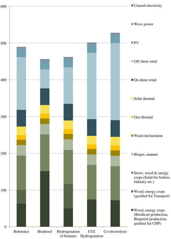
Figure 49. Primary energy supply in the 2050 reference energy system and analysed scenarios
