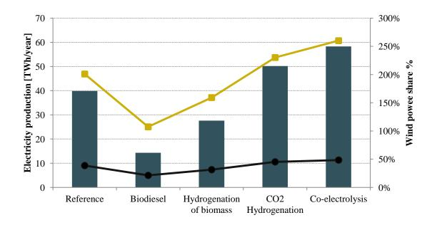
Figure 48. Off-shore electricity production (columns, TWh/year) with according share of total wind power in primary energy supply (black line, %) and wind share of projected electricity demand (yellow line, %)
