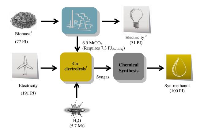
Figure 30. Co-electrolysis scenario. <sup>1</sup>Based on dry willow biomass. <sup>2</sup>Assumed an electricity generation efficiency of 40%. <sup>3</sup>Assumed an electrolyser efficiency of 78% [67], minus 5% account for storage and chemical synthesis losses.
