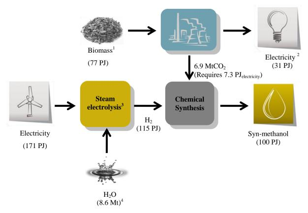
Figure 31. <sup>1</sup>Based on dry willow biomass. <sup>2</sup>Assumed an electricity generation efficiency of 40%. <sup>3</sup>Assumed an electrolyser efficiency of 73% [12], minus 5% account for storage and chemical synthesis losses. <sup>4</sup>This does not include the excess water which can be recycled from the hydrogenation process.
