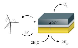
Figure 25. Solid oxide cell water electrolysis
