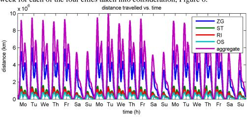
Figure 6 Output from MATSim: time series of kilometres driven for three weeks
