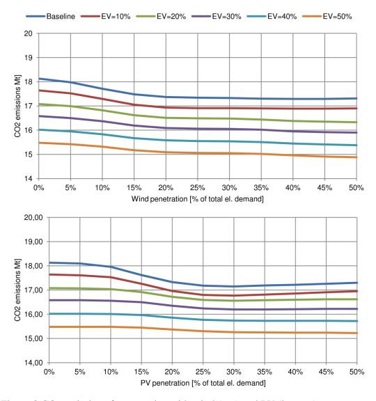
Figure 8 CO<sub>2</sub> emissions for scenarios with wind (top) and PV (bottom)
