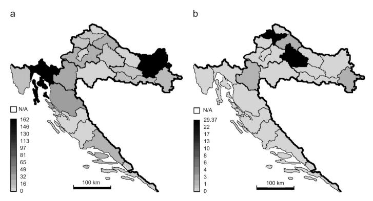
Fig. 6. (a) Energy capability of potential biomass facilities (GWh) and (b) maximum load capacity of potential geothermal facilities (MW).
