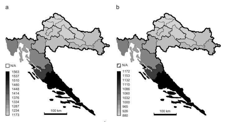
Fig. 2. (a) Global horizontal irradiation (kW h/m<sup>2</sup>/year) and (b) PV power (horizontal) (kW h/year for 1 kW p).
