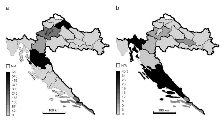
Fig. 7. Energy capability (GWh) of potential: (a) large and (b) small hydro power plants.
