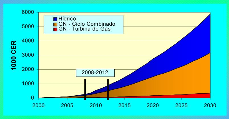
CDM potential: comparison of scenarios to the baseline - gas turbine natural gas, combined cycle natural gas, hydro
