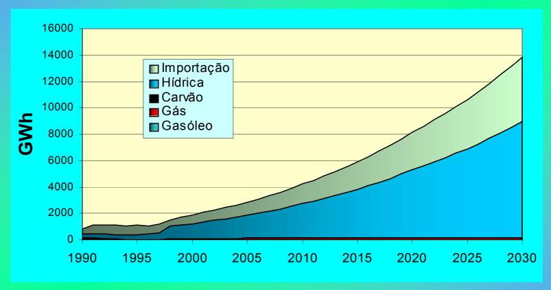
Hydro scenario: electricity production (hydro + coal + natural gas + Diesel) and import
