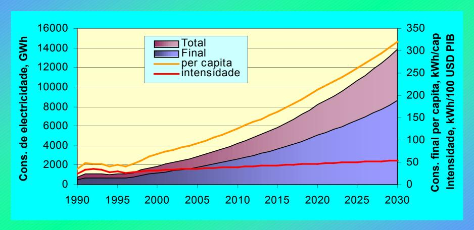
Baseline scenario: Total and final electricity consumption, per capita electricity consumption and electricity intensity
