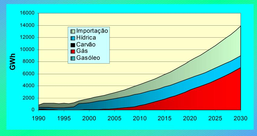
Natural gas scenario: electricity production (hydro + coal + natural gas + Diesel) and import
