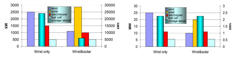
For peak shaving wind&solar takes smaller storage and electrolyser
